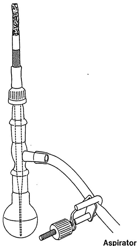
**Figure 6.1.** Apparatus used to trap cigarette smoke. (Adapted from Leanderson and Tagesson, 1989).
