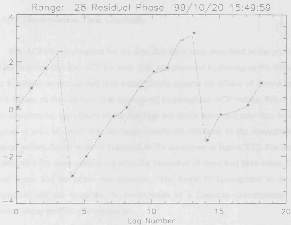
Figure 7.10: An ACF obtained during the longer lag mode. As for the ACF corresponding to natural irregularities shown above, this ACF now decorrelates indicating an irregularity distribution that is not static for the longer sampling time.
