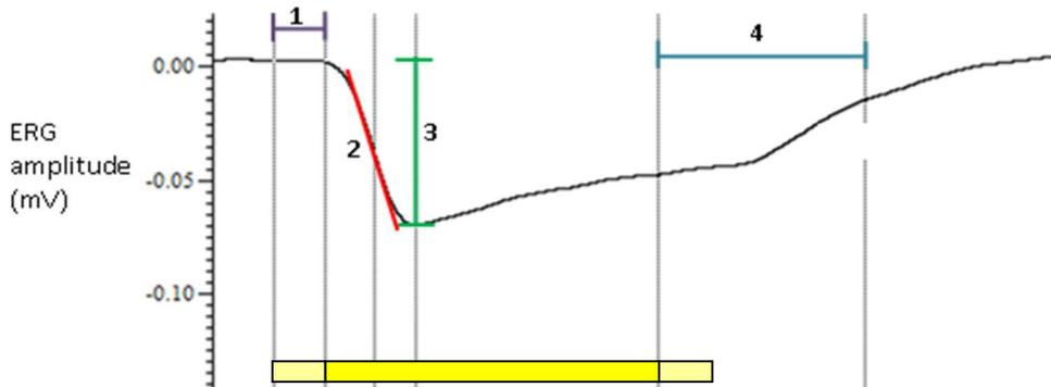
Figure 15: (as in Figure 8B) Example of typical electroretinogram trace with measures shown. Purple (1): latency; Red (2): maximal slope; Green (3): maximal response amplitude; Blue (4): 50% repolarisation time. Yellow bar indicates light pulse (faded yellow indicates transition)
