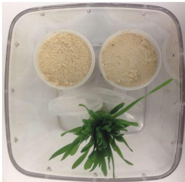
Figure 3: Example layout of emergence experiment (top view). The tubes were continuously recorded, with low level red light in addition to the cycling white light cycle. Container measured 110 x 110 mm at the widest points and was aerated with small holes (approx 1 mm diameter) around the top.
