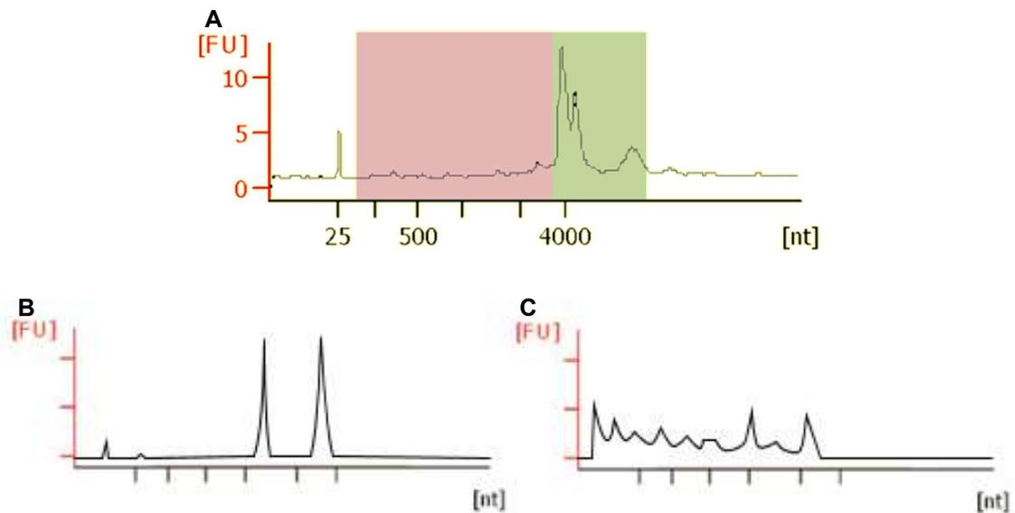
**Figure 6: Example electropherograms. Sample G16B (A). Ideal high quality sample (B) and highly degraded sample (C). Both B and C represent hypothetical mammalian samples so the exact location of the ribosomal peaks differs from *S. gregaria*. Axis units, X: nucleotides (nt), Y: fluorescence units (FU). Sharp peaks in the green region represent ribosomal RNA and are indicative of high quality RNA as in B; peaks in the red region would indicate degradation of the ribosomal RNA as in C.**
