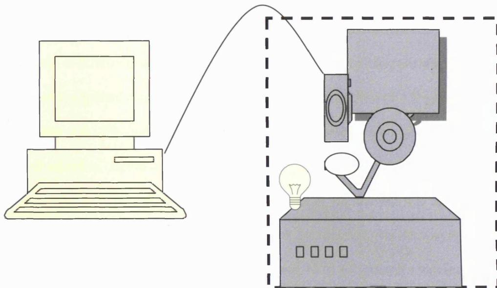
**Figure 4.3.** Monitoring CAM microcirculation using intravital microscopy. A clear Perspex incubator was constructed around the video microscopy camera and lighting.
