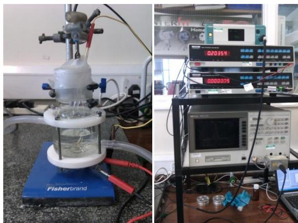
**Fig. 3.3** - Jacketed electrochemical quartz crystal microbalance cell (left hand image) and instrument set-up (right hand image).
