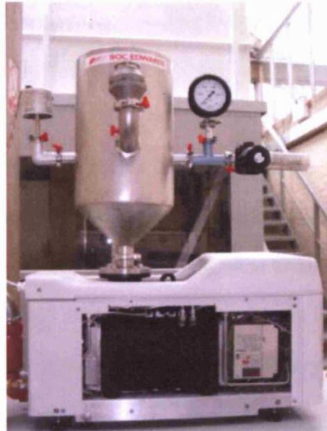
Figure 2-2: The iGX dry vacuum pump test-bed
