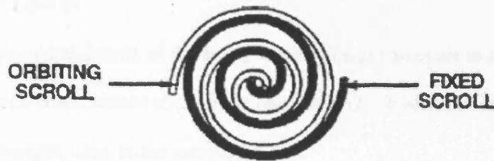
Figure A-3: Scroll type design (adapted from Lessard [Lessard 2000])
