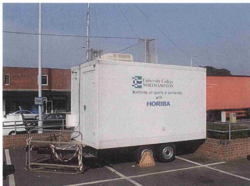
Figure 3.3: Fixed-site air pollution monitoring unit at the roadside location in Kingsthorpe, Northampton.
