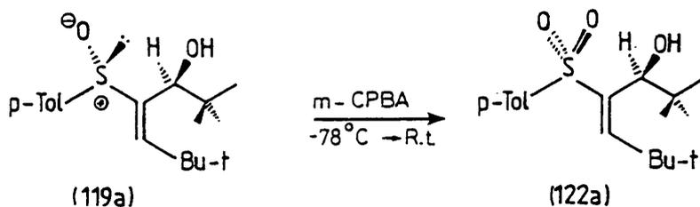
The optical rotation was measured at  $-20.8^{\circ}$  (2.0 in  $\text{CHCl}_3$ ) confirming that (122a) and (122b) were enantiomeric and that the diastereomeric sulphinyl allylic alcohols (119a) and (119b) had opposite configurations at the chiral carbon atom.
