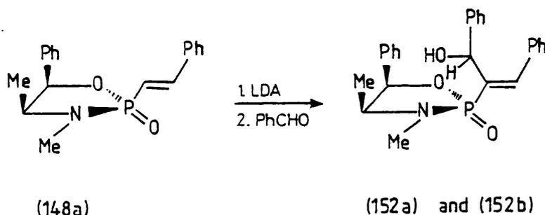
However, the reaction was not deemed a success because the diastereomeric ratio was measured at 1:1.18, with a total yield of (152a) and (152b) of only 35% and separation by flash chromatography on a silica gel column resulting in partial decomposition of the products.
