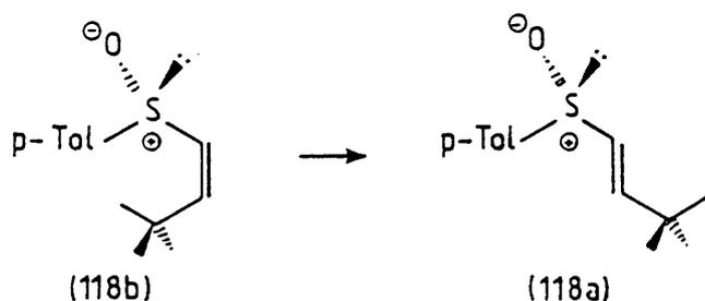
Using the same procedure as for the deprotonation of (53a),<sup>1</sup> (Z)-3,3-dimethyl-1-[(R)-p-tolylsulphinyl]-1-butene (118b) (100 mg, 0.45 mmol) was deprotonated with LDA (0.63 mmol) and after 1h quenched with a 1:1 water/THF mixture. T.l.c. showed the complete disappearance of the (Z)-starting material and after work-up and purification by 'chromatotron' (ether), (E)-3,3-dimethyl-1-[(R)-p-tolylsulphinyl]-1-butene (118a) was obtained as a white solid<sup>2</sup> (70 mg, 70%).
