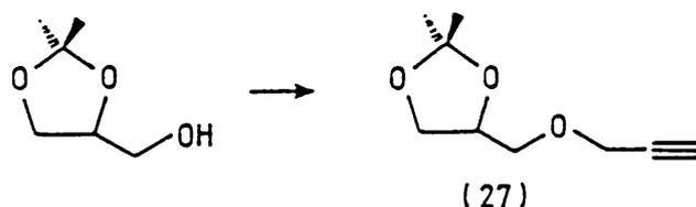
Using the same procedure as for the preparation of (22),<sup>1</sup> 1,2-O-isopropylidene-1,2,3-trihydroxypropane<sup>2</sup> (10g, 76 mmol) in DMF (15 ml) was added to sodium hydride (2.28g, 76 mmol) in DMF (20 ml)<sup>3</sup> and quenched with propargyl bromide (8.4 ml, 76 mmol) in DMF (10 ml). Work-up afforded a brown oil which after Kugelrohr distillation (ca. 16 mmHg) gave 1,2-O-isopropylidene-1,2-dihydroxy-3-(2-propynyl-1-oxy)-propane (27) as a colourless liquid (5.8g, 45%).
