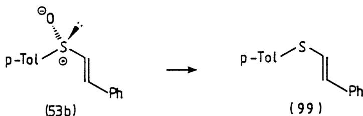
Using the same procedure as for the reduction of (94a)<sup>1</sup> (+)-(E)-2-phenyl-1-[(R)-p-tolylsulphinyl]-ethylene (53b) (108 mg, 0.45 mmol) was reduced by aluminium amalgam (120 mg, 4.4 mmol) in 4h. After work-up and removal of solvent in vacuo, the crude white solid was purified by 'chromatotron' (petroleum ether) to give (E)-2-phenyl-1-(p-tolylthio)-ethylene (99) as a white solid (85 mg, 84%).
