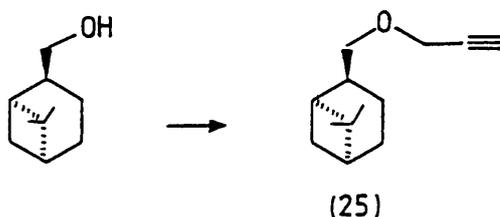
Using the same procedure as for the preparation of (22),<sup>1</sup> (-)-trans-myrtanol (2.07 ml, 13 mmol) was added to sodium hydride (0.39g, 13 mmol) in DMF (15 ml) and quenched with propargyl bromide (1.3 ml, 11 mmol) in DMF (3 ml). Work-up afforded a brown viscous oil which after distillation (170°C at 0.4 mmHg) and flash chromatography (19:1 petroleum ether-ether) gave 3-myrtoxypropyne (25) as a colourless oil (0.94g, 38%).
