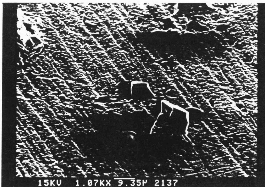
Figure 8.15: SEM of the Deposit Formed by the Reaction of  $\text{RuF}_5$  and  $\text{H}_2$  at  $250^\circ\text{C}$
