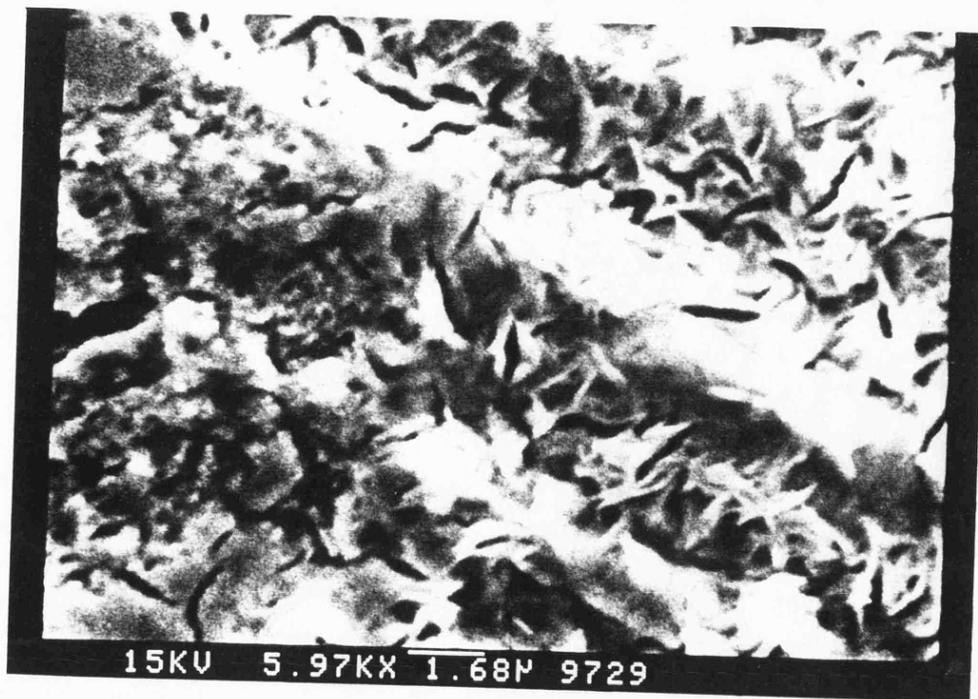
Figure 8.8: SEM of the Deposit Formed by the Reaction of  $\text{UF}_6$  and  $\text{H}_2$  at  $175^\circ\text{C}$
