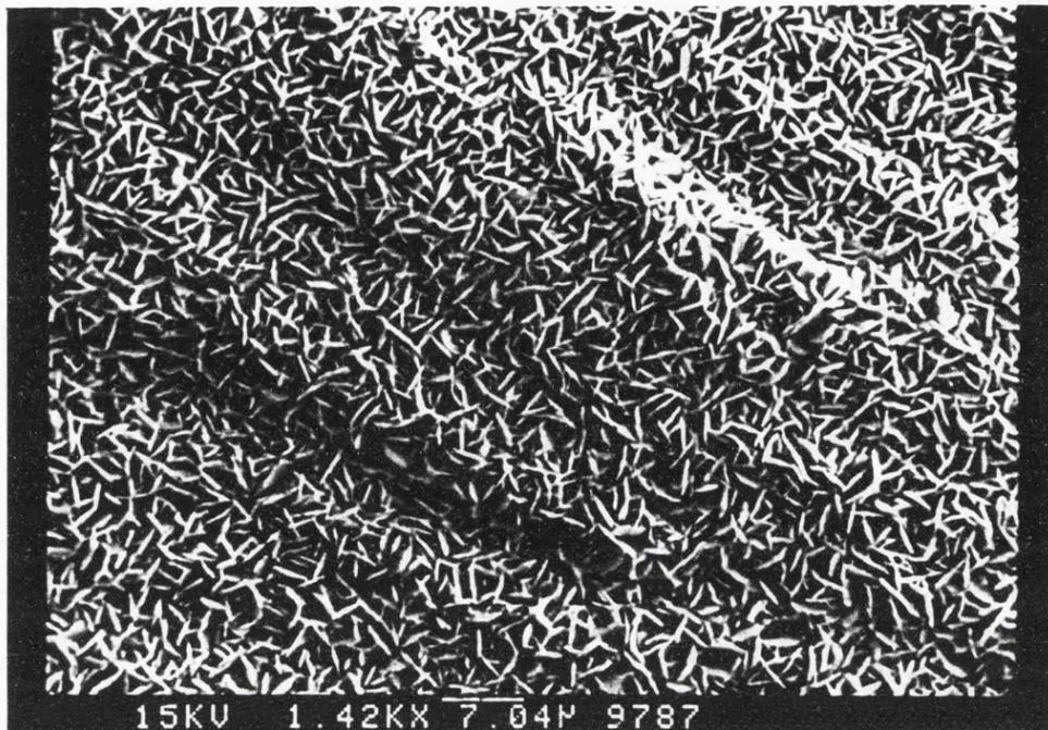
Figure 8.9: SEM of the Deposit Formed by the Reaction of  $\text{UF}_6$  and  $\text{H}_2$  at  $200^\circ\text{C}$
