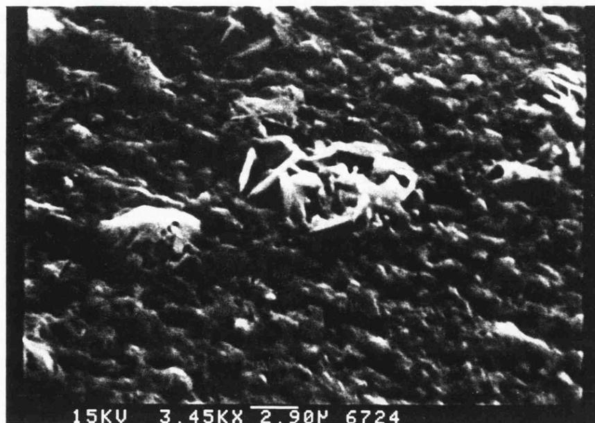
Figure 8.10: SEM of the Deposit Formed by the Reaction of  $\text{UF}_6$  and  $\text{H}_2$  at  $250^\circ\text{C}$
