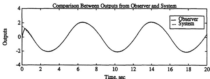
Figure 3.1: Comparison between outputs from the observer and system
