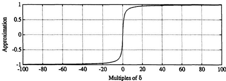
Figure 2.5: A differentiable approximation of the *signum* function
