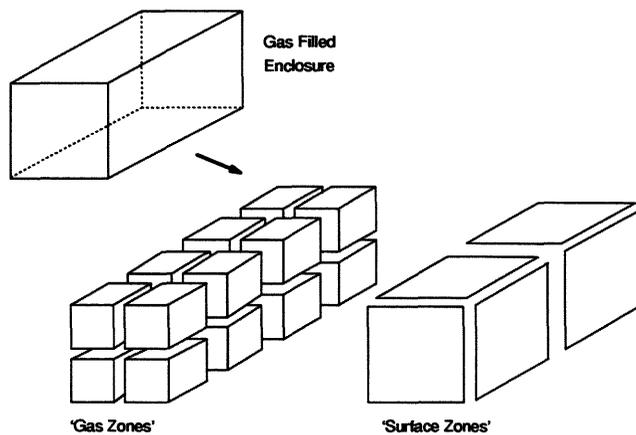
Figure 6.5: Schematic of the Zone Method
