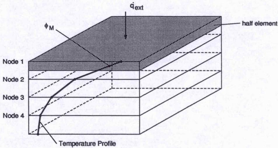
Figure 6.4: Half element at the surface
