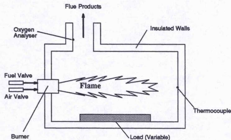
Figure 6.1: Schematic of the furnace considered
