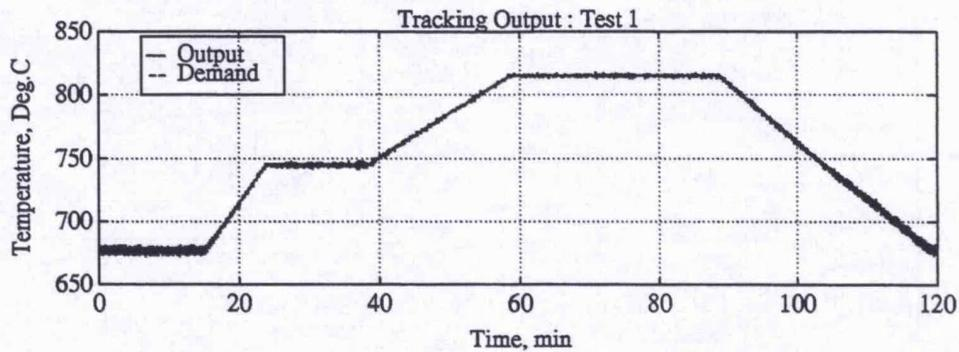
Figure 7.7: Experimental furnace under PID Control
