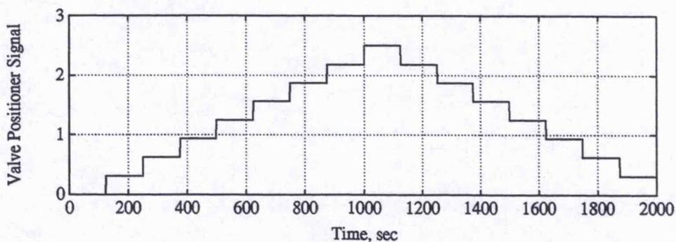
Figure 6.8: Valve positioner excitation signal
