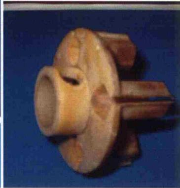
Static shaft for EXTPMFSM 2    Plastic stator lamination frame for EXTPMFSM 2
