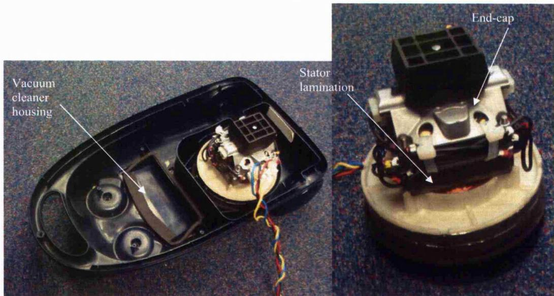
Figure 4.5: Photo of actual polygon-shaped flux switching motor with supports
