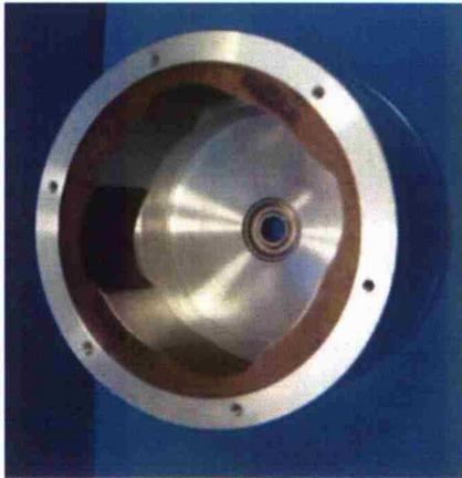
Rotor lamination and frame assembly for EXTPMFSM 2
