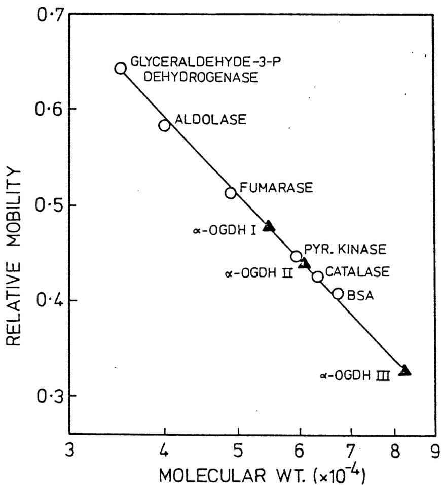
Fig. 19. Dependence of log molecular weight on the relative mobility after polyacrylamide gel electrophoresis in the presence of sodium dodecyl sulphate. SDS gel electrophoresis was performed using standard proteins of known molecular weight and A. lwoffii  $\alpha$ -OGDH complex, as described in section II.2.9.
