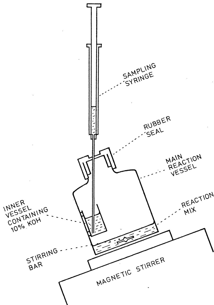
Fig. 7. The reaction vessel used for radiochemical assays
