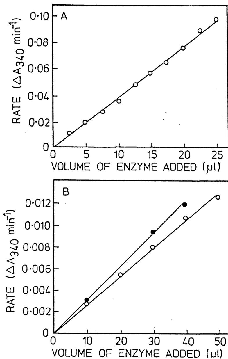
Fig. 14. Dependence of the observed rate on the concentration of dihydrolipoamide transacylase (E2).
