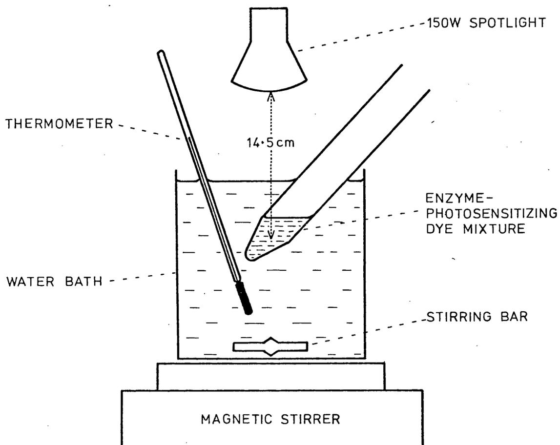
Fig. 31. Apparatus used for photooxidation.
