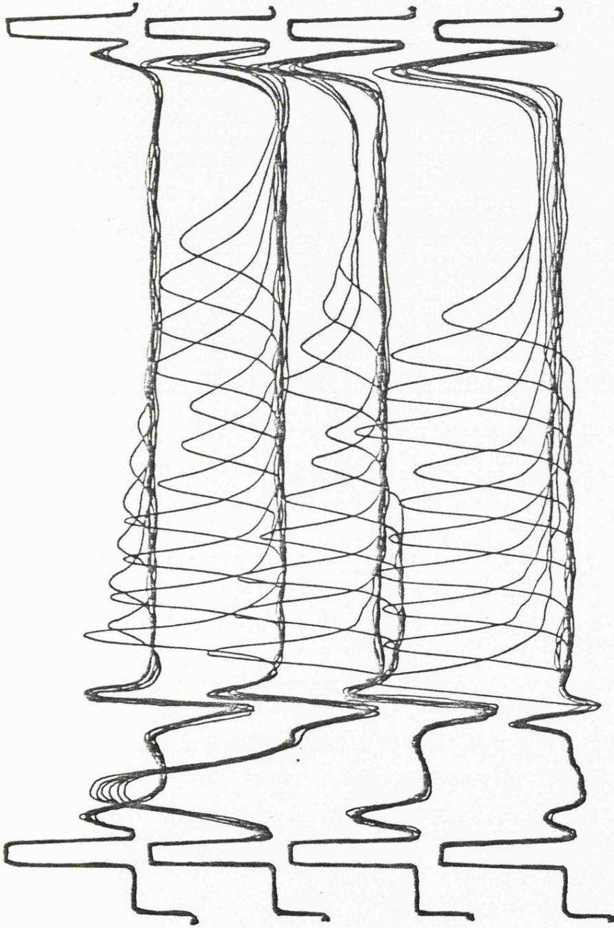
Fig. 20. Sedimentation analysis of purified  $\alpha$ -OGDH complex from A. lwoffii. Samples of  $\alpha$ -OGDH ( $2.56, 5.13, 6.83$  and  $10.25\text{mg ml}^{-1}$  in  $0.1\text{M Tris-HCl}$ , pH  $8.0$  containing  $8\%$  glycerol) were sedimented at  $40,000\text{rpm}$  at  $5^{\circ}\text{C}$  in an MSE Centrifuge  $75$  ultracentrifuge using Schlieren optics to observe the boundary position at suitable time intervals. Experimental details are given in section II.2.10.
