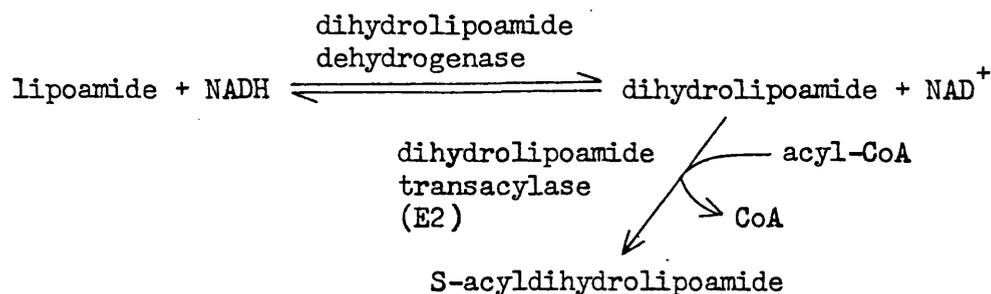
An excess of exogenous dihydrolipoamide dehydrogenase is allowed to act on oxidized lipoamide and NADH and thereby produce an equilibrium mixture of lipoamide, dihydrolipoamide, NADH and  $\text{NAD}^+$ . After introducing E2 enzyme and the appropriate acyl-CoA, dihydrolipoamide is removed by acylation. The rapid establishment of an equilibrium by the dihydrolipoamide dehydrogenase allows this removal to be monitored continuously by following the oxidation of NADH at 340nm.
