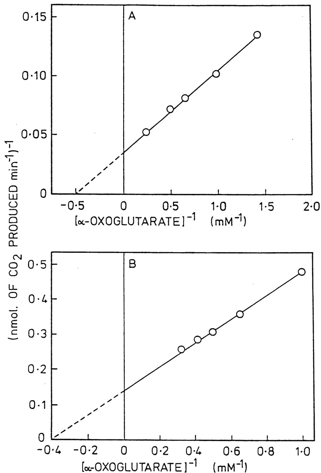
Fig. 13. Determination of the  $K_m$  for  $\alpha$ -oxoglutarate using the EI and whole complex radiochemical assays.
