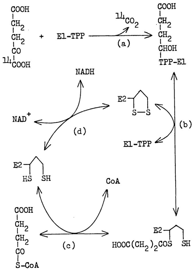
Fig. 5. The reaction sequence of the  $\alpha$ -OGDH complex showing the release of  $[\text{}^{14}\text{C}]\text{CO}_2$  from  $[\text{}^{1-}\text{}^{14}\text{C}]\alpha$ -oxoglutarate.
