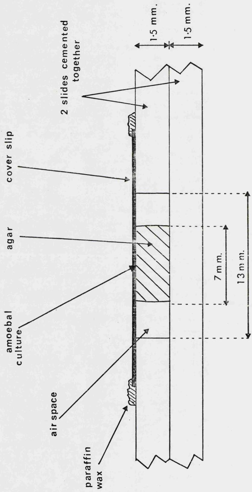
Figure 8. Longitudinal section through the central part of a filming slide to show the culture chamber.
