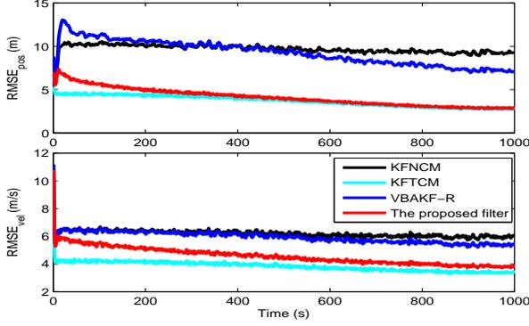
Fig. 1: RMSEs of the position and velocity.
