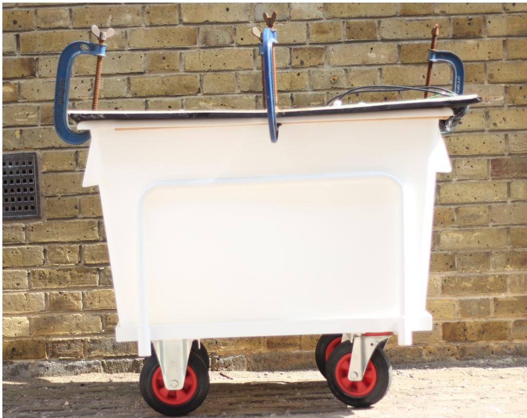
Figure 2.2 Image of the chamber developed for the study of decomposition VOCs associated with pig carcasses
