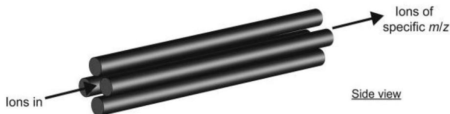
**Figure 5:1** Diagram of a quadrupole mass analyser adapted from Ellis and Mayhew (2014a)
