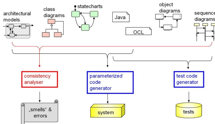
Figure 2 – UML/P used for code and test generation.
