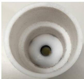
**Figure 3.6.** An image of the Teflon cell used with a quartz crystal in the centre of it
