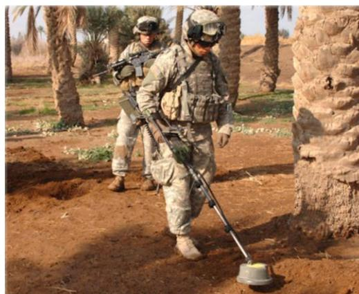
Figure 2-6. The AN/PSS-14 Hand-held landmine detection sensor [42].
