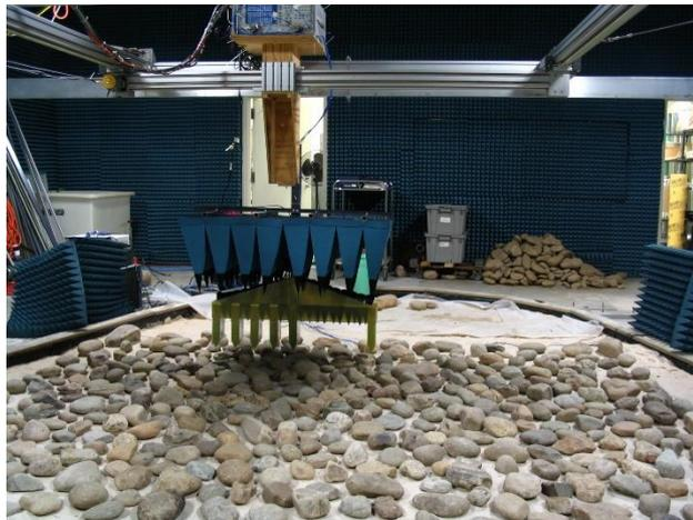
Figure 2-7. GPR array from the Wrocott research group [43].
