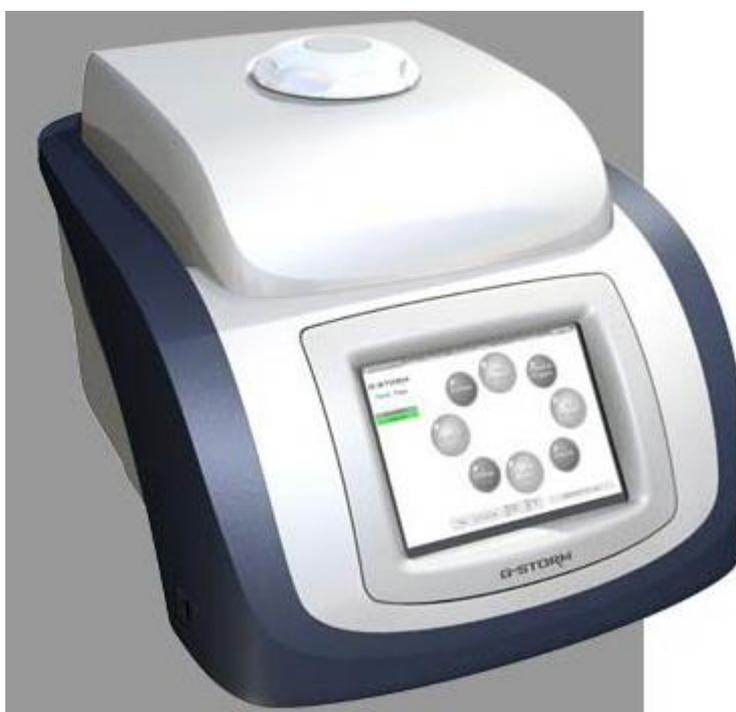
Figure 7.9: The GS1 Thermal Cycler: Utilised to Perform PCR reactions.
