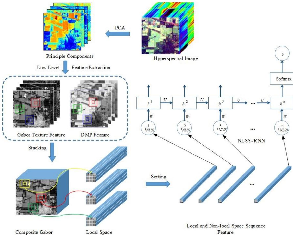
Fig. 1. The framework of the proposed NLSS-RNN method.
