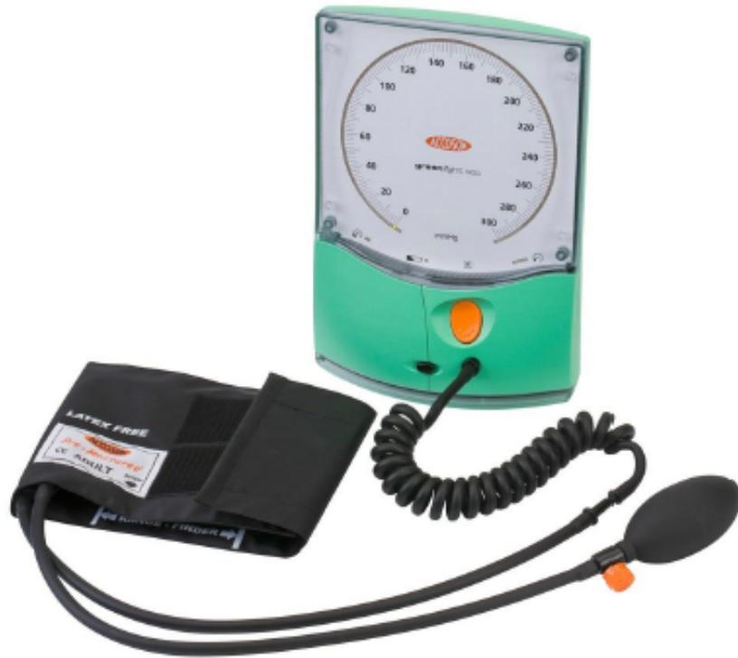
**Figure 2.2. The Accoson Greenlight 300.** A mercury-free manual sphygmomanometer.
