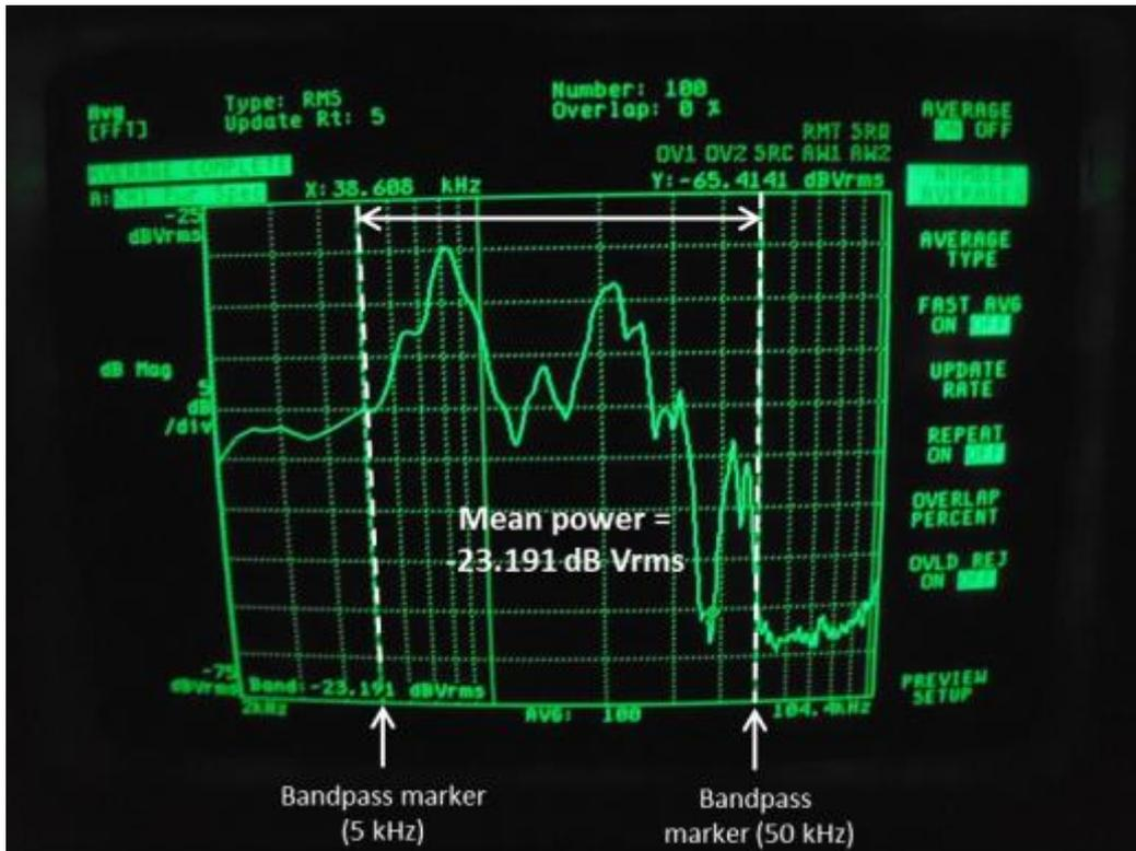
**Fig 8.5. Average power spectrum of broadband noise generator.** A signal analyser (Agilent HP3566A Dynamic Signal Analyser) was used to calculate the average power spectrum (100 sweeps) of the noise generated by the ‘acoustic overexposure set-up’ at a calibrated distance from the speaker (20 cm) within a sound attenuated booth. Bandpass markers were set between 5 and 50 kHz, with the mean power of signal falling between the bandpass markers measured at -23.191 dB Vrms (equal to 107.8 dB SPL)
