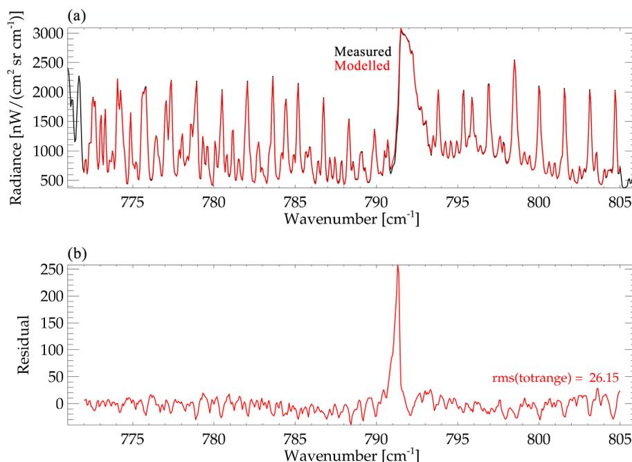
**Figure 4.** Impact of the CO<sub>2</sub> Q-branch at 11.5 km altitude without considering line mixing: (a) spectra; (b) residuals. Black: measured spectrum, hardly discernible because overplotted by modelled spectra.
