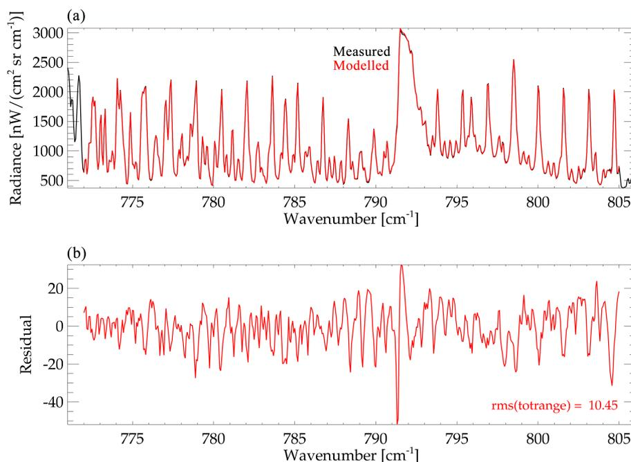
**Figure 5.** Impact of the CO<sub>2</sub> Q-branch at 11.5 km altitude taking line mixing into account: (a) spectra; (b) residuals. Black: measured spectrum, hardly discernible because overplotted by modelled spectra. Note the different scale of the residual axis compared to Fig. 4.
