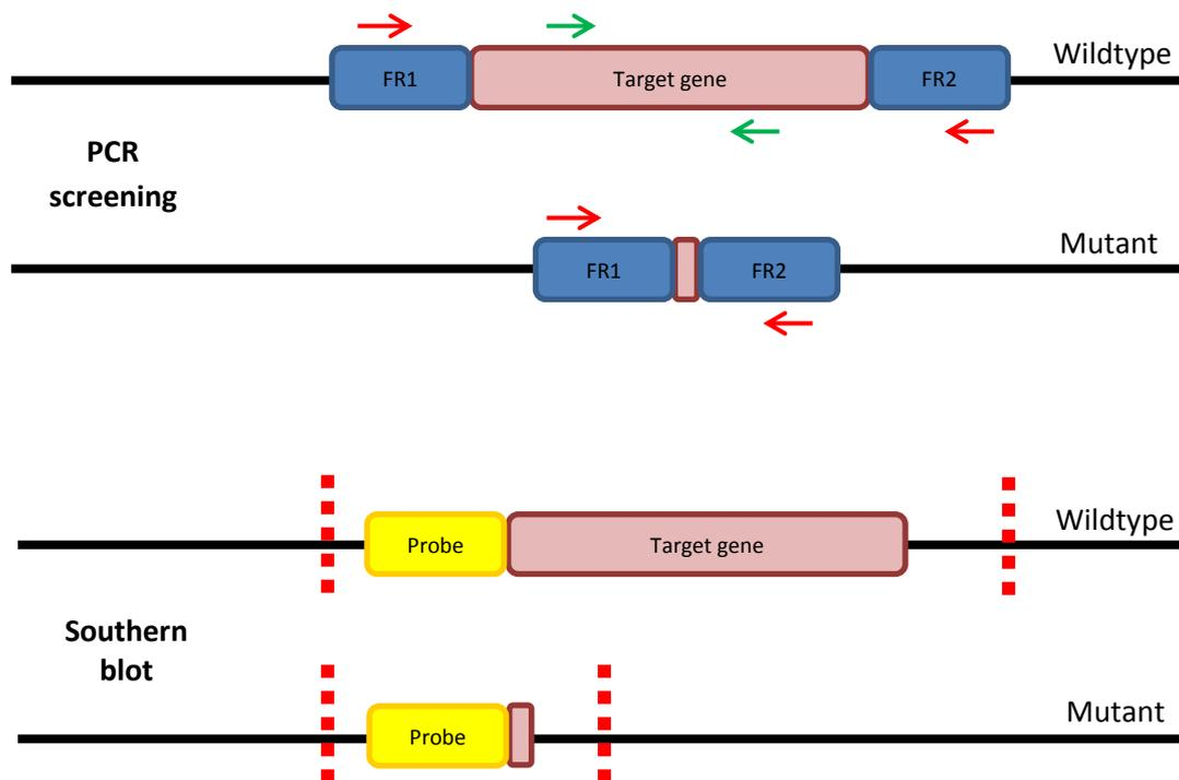
**Figure 23: Schematic of PCR and Southern blot screening of deletion mutants.**
