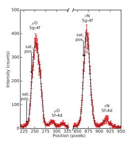
**Figure 4.** Simultaneously measured spectra of 5g-4f transitions in muonic oxygen (energy calibration) and pionic nitrogen. The parallel transitions 5f - 4d and possible additional transitions from the presence of one remaining electron in the K shell are indicated ("sat. pos."). For  $\mu$ O, the larger width of the 5g - 4f transition is due to the non-resolved fine structure splitting, which is resolved for the 5f - 4d transition.
