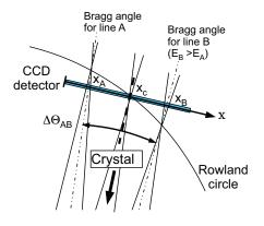
**Figure 5.** Scheme of the X-ray detector position with respect to the Rowland circle (the focus location of the spectrometer) and two diffracted lines *A* and *B* with different energy  $E_B > E_A$ . The (small) displacements of the two lines from their individual focal conditions is taken into account in the calculation of the spectrometer response by means of a Monte-Carlo ray tracing calculation.
