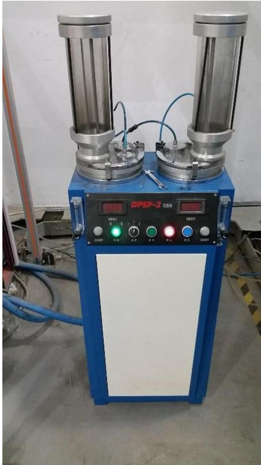
*Figure 35 - Containers for the alloyed powders to be blown at the nozzles.*
