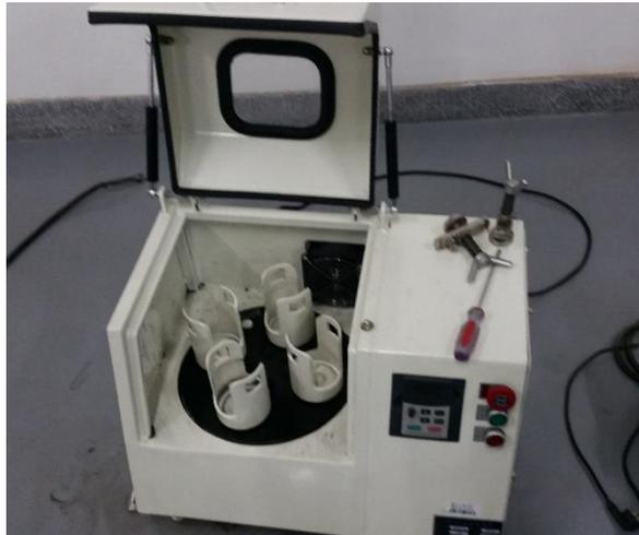
*Figure 34 - MITR YXQM-0.4 L ball mill used in the mixture of elemental powders.*
