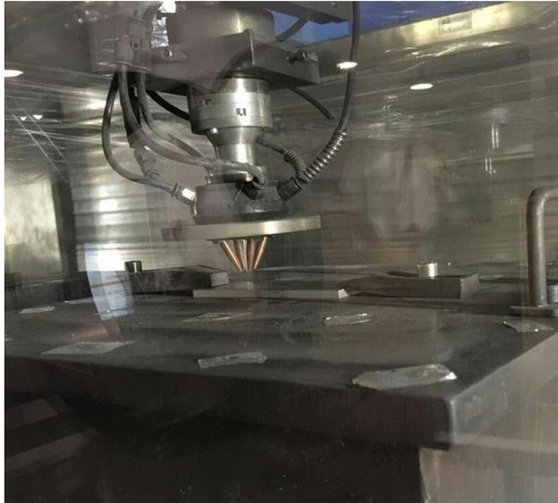
Figure 36 - LSF-SI600A model laser additive manufacturing machine used for the experiments.
