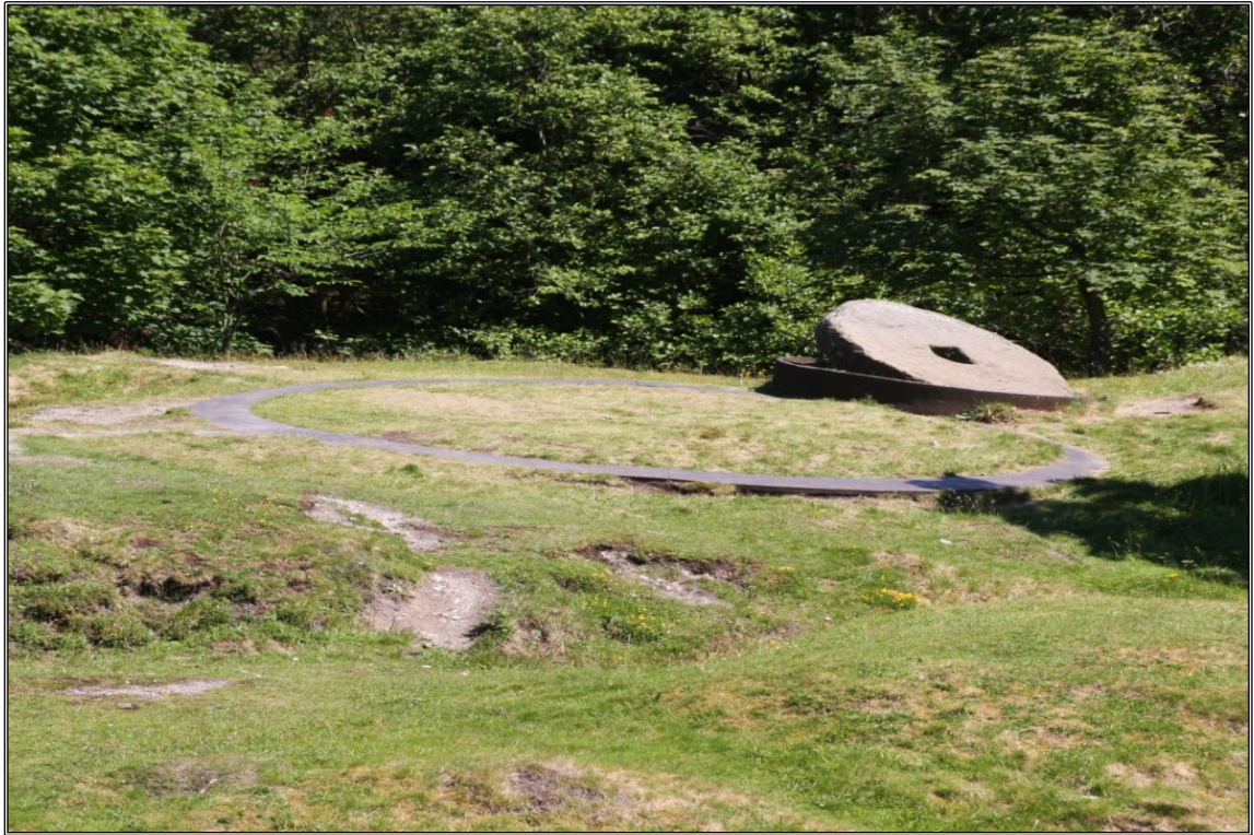
Figure 3.11. Lead ore crushing circle near the Odin mine. This is a reconstruction west of Castleton, Derbys. The grindstone was tethered by a pole to the centre of the circle and towed round the circle by animal or hand. SK 141 842 (Photograph by CS, 2010.)
