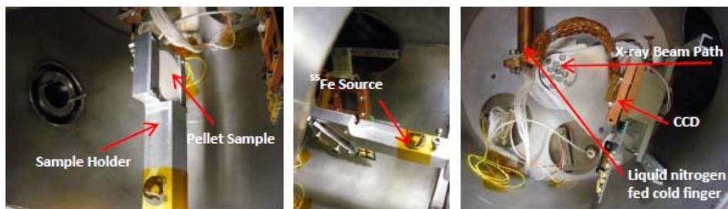
**Figure 3.9.** Photographs of the pre-existing CCD facility showing where the X-ray beam enters the vacuum chamber, position of the CCD and the pellet sample holder with the  $^{55}\text{Fe}$  source secured on the side.
