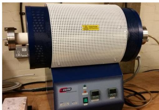
Figure 24: Shows tube furnace used for heat treatment of Nb-Si-Ti alloys
