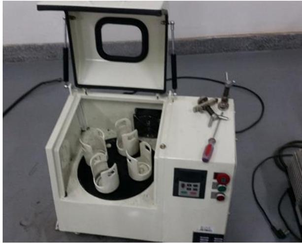
Figure 17: Ball mill used to grind powders to even size
