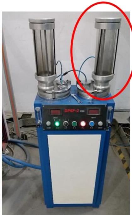
Figure 18: DPSF-2 container (highlighted) used to store powder before processing
