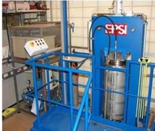
Figure 23: Shows the HIP equipment used during experiments<sup>[92]</sup>
