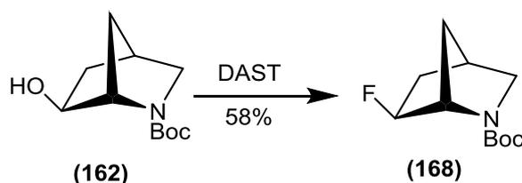
**Fig. 3.15** The overall synthesis of 2-Boc-6-*exo*-fluoro-2-azabicyclo[2.2.1]heptane (yield of isolated compound).
