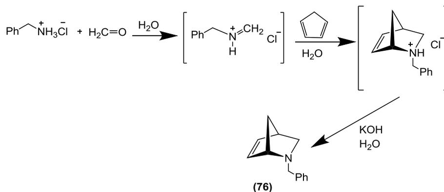
**Fig. 2.7** Synthesis of 2-benzyl-2-azabicyclo[2.2.1]hept-5-ene through aqueous hetero Diels-Alder reaction.
