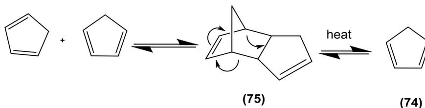
**Fig. 2.6** Retro Diels-Alder reaction to produce cyclopentadiene.
