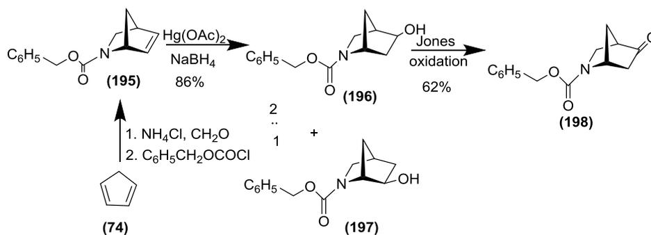
**Fig. 4.4** Carroll methodologies which describe the conversion of cyclopentadiene to 2-(Carbobezyloxy)2-azabicyclo[2.2.1]heptan-5-one (**198**).<sup>164</sup>
