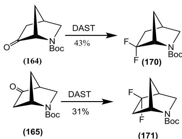
**Fig.3.18** The overall synthesis of 2-Boc-6,6-difluoro-2-azabicyclo[2.2.1]heptane and 2-Boc-5,5-difluoro-2-azabicyclo[2.2.1]heptane (yields of isolated compounds).
