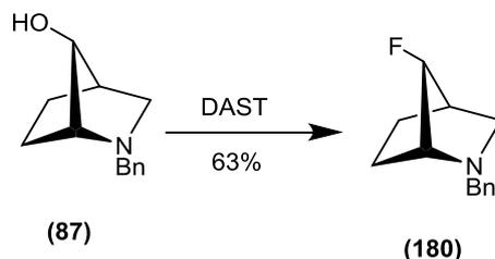
**Fig. 3.25** The synthesis of *anti*-7-fluoro-2-benzyl-2-azabicyclo[2.2.1]heptane (**180**).
