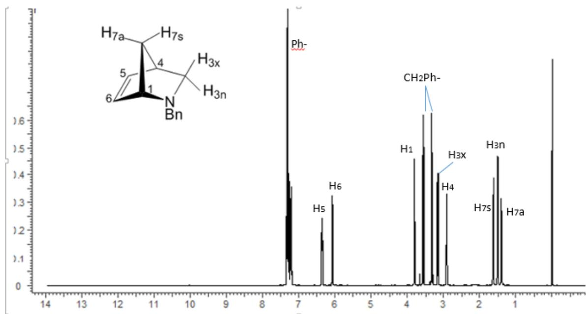
**Fig. 8** The  $^1\text{H}$  NMR spectrum of the 2-benzyl-2-azabicyclo[2.2.1]hept-5-ene (**76**).
