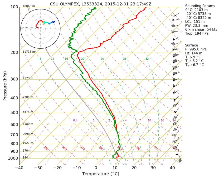
**Figure 1.** Skew-T log-P diagram of the atmospheric temperature (continuous red line) and dew-point temperature (continuous green line) profiles from the Rawinsonde sounding launched at NPOL site on 1 December 2015, at 2317 UTC (extracted from <http://olympex.atmos.washington.edu/archive/reports/20151201-2/soundings/research.skewt.201512012300.csu.png>). NPOL = NASA S Band Dual-Polarimetric Radar; OLYMPLEX = Olympic Mountain Experiment.
