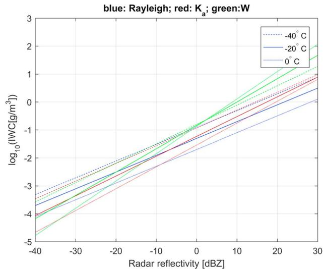
**Figure 8.** Empirical formula relating ice water content (IWC) to temperature and  $Z_e$  measured by a Rayleigh (blue), Ka (red), and W band (green) radar from Hogan et al. (2006) and Protat et al. (2007).
