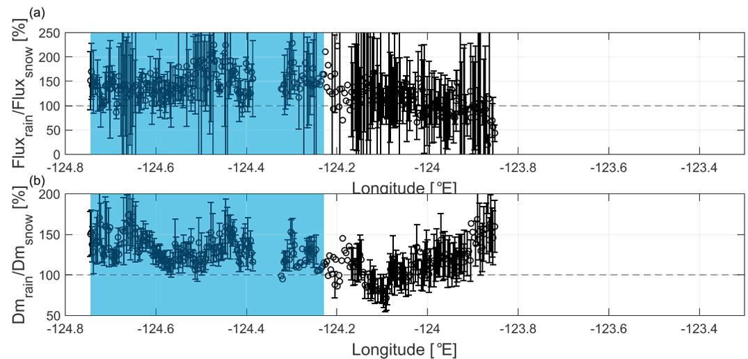
**Figure 15.** (a) Ratio between the rain flux and snow flux retrieved just above and below the melting layer. (b) Ratio between the rain  $D_m$  and the snow melted  $D_m$  retrieved just above and below the melting layer.
