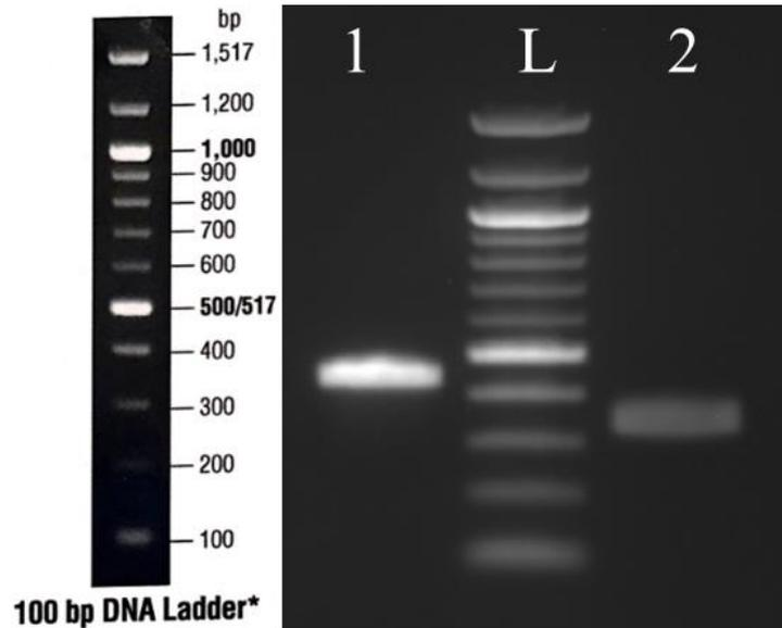
**Figure 3.21.** Agarose gel electrophoresis illustrates the amplified upstream regions containing the putative promoter regions of the target genes. L: 500 ng of 100 bp DNA ladder (NEB). Lanes 1-2: putative promoter regions of *rgg0999* (430 bp), and *rgg1518* (327 bp), respectively.
