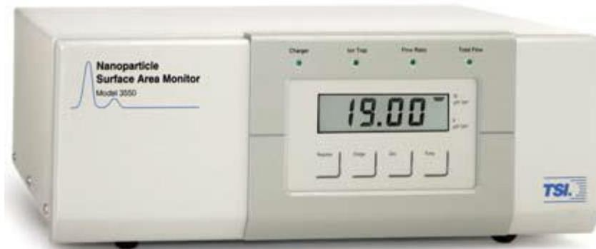
Figure 2.14: Nanoparticle surface area monitor TSI 3550.
