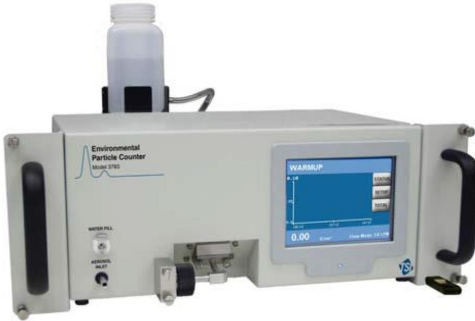
Figure 2.8: Model 3783 Environmental Particle Counter.
