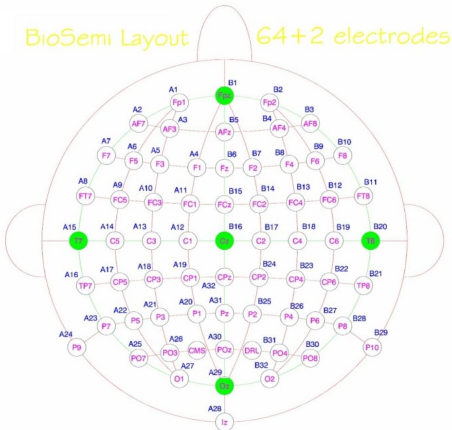
**Figure 2.3 Biosemi Active-Two 64-Channel EEG:** The layout of the 64 channel electrodes on the scalp. The nose and the front of the head are at the top of the figure.
