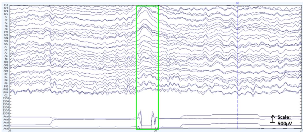
**Figure 1.3 Segment of all EEG channels for one subject showing eye movements:** On the left are the labels for each channel. And the raw signal from the EEG (top section) is shown in navy blue. There are also the eye tracker signals shown (at the bottom section), which also have traces in navy blue. The green box surrounds an eye movement called a blink.
