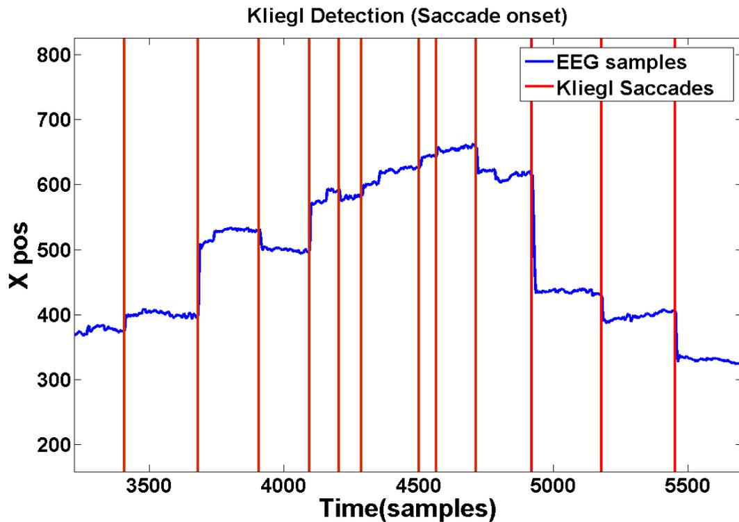
**Figure 2.16 Kliegl saccade detection algorithm:** The blue trace is the x-axis position of the eye from the EEG eye trace. The vertical red lines are the times the Kliegl algorithm detected a saccade.
