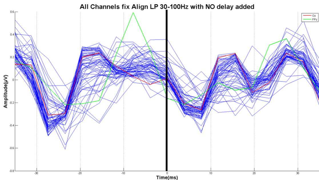
**Figure 2.12 Fixation aligned fRP filtered between 30-100Hz:** Here are all the channels across the scalp with FPz highlighted in green and the Oz electrode highlighted in red. The black vertical line shows  $t=0$ .
