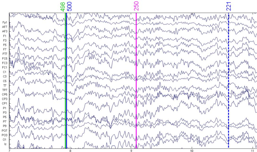
**Figure 2.7 Example of triggers being sent to the EEG trace shown:** Different channel traces are shown in the navy blue each labelled in the y-axis. The vertical coloured lines are different triggers that can be sent to the EEG to show events that occurred at a point in time during an EEG experiment.
