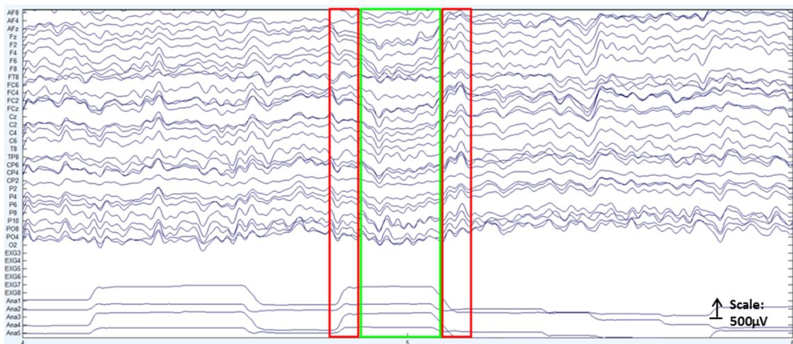
**Figure 1.2 Segment of all EEG channels for one subject showing eye movements:** On the left are the labels for each channel. And the raw signal from the EEG (top section) is shown in navy blue. There are also the eye tracker signals shown (at the bottom section), which also have traces in navy blue. The two red squares surround an eye movement called a saccade and the green box surrounds an eye movement called a fixation.
