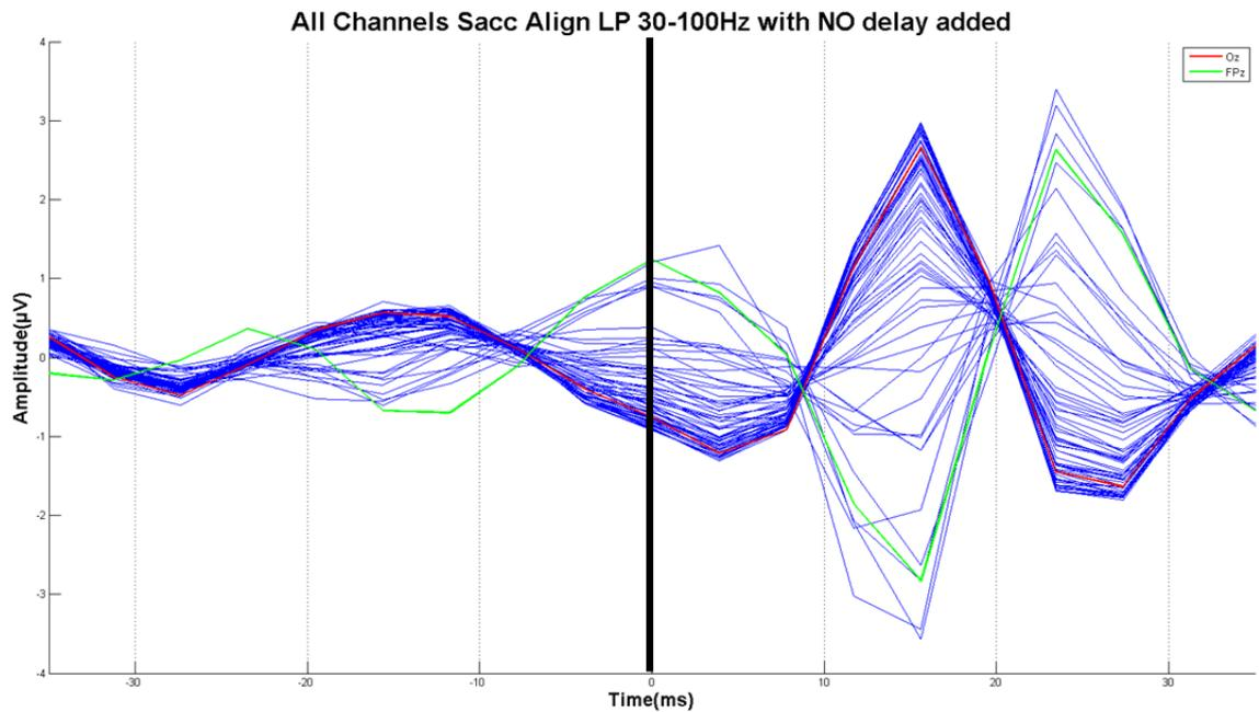
**Figure 2.13 Saccade aligned sRP filtered between 30-100Hz:** Here are all the channels across the scalp with FPz highlighted in green and the Oz electrode highlighted in red. The black vertical line shows  $t=0$ .
