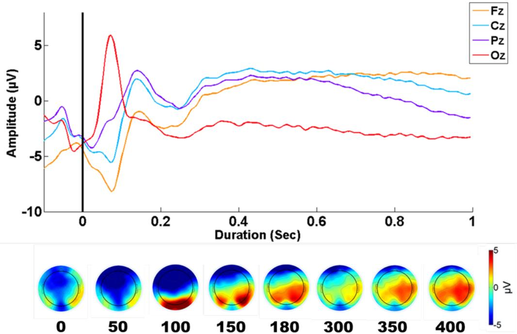
**Figure 4.20 Activity at the onset of the target: Top panel:** The averaged fRP, focussing on the target fixation between  $[0.1\ 1]$  seconds. The four midline electrodes are shown again; Fz (orange), Cz (cyan), Pz (purple) and Oz (red). **Bottom panel:** show the topographies of the activity shown in the top panel from  $[0\ 400]$  ms the sequence of steps is highlighted below.
