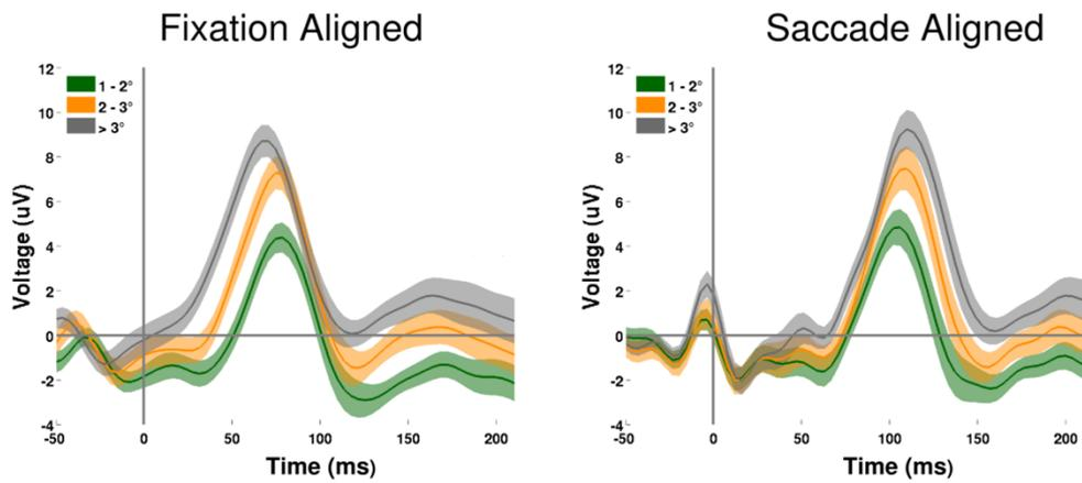
**Figure 2.10 Noticing a signal processing issue:** Two different alignments of the P100 potential at the Oz electrode are shown; fixation-aligned (left hand side) and saccade-aligned (right hand side). Each trace are the grand average potentials isolated for saccade size. Saccades of sizes 1-2° (green), 2-3° (orange) and >3°.
