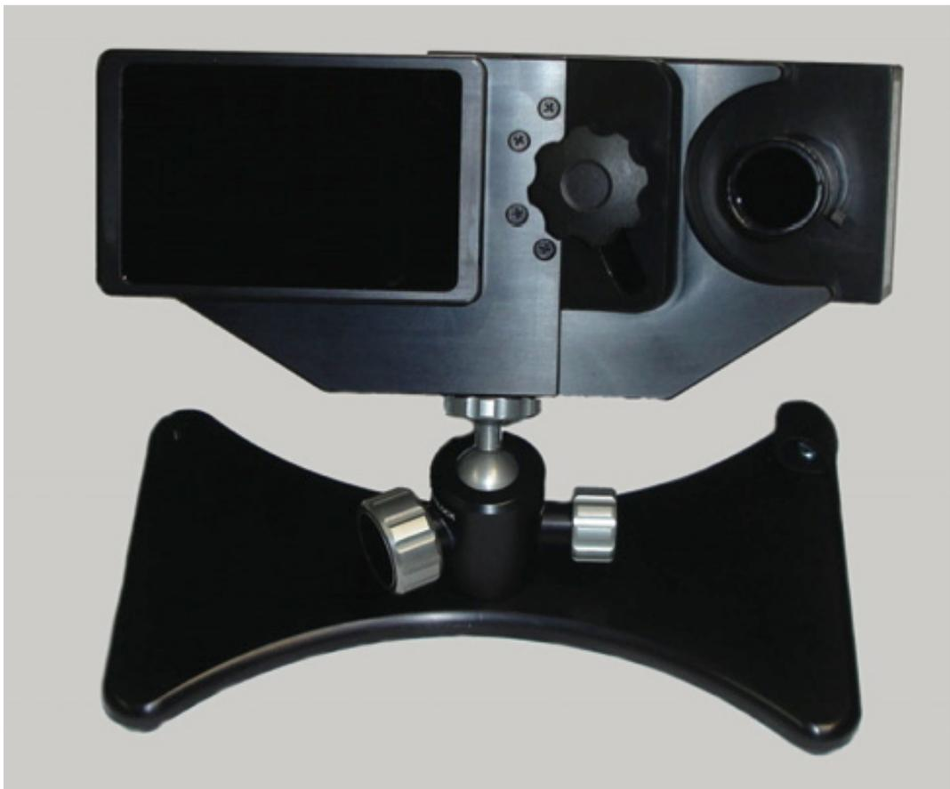
**Figure 2.4 Eyelink 100 Eye-Tracker:** The eye tracking hardware, on the left is a light board made of infrared LEDs and on the right is the high resolution camera.
