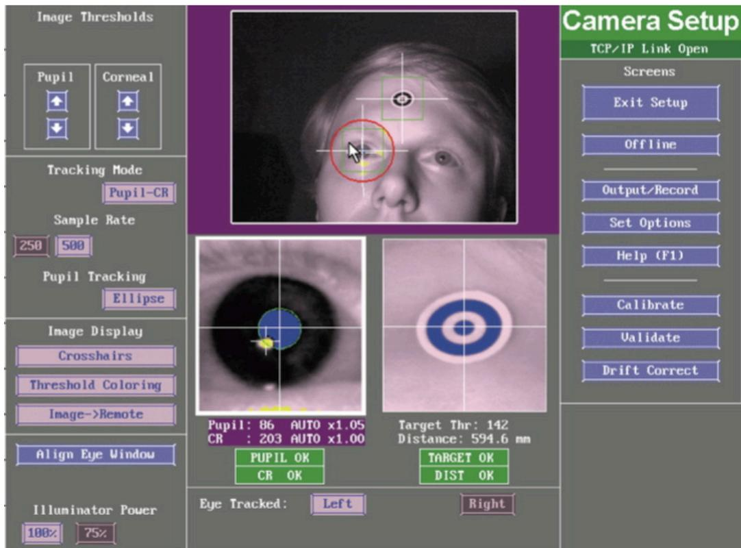
**Figure 2.5 Eyelink 100 software:** The software used to collect the eye movements. On the screen is an example of the eye tracker software. On the right there are the different options to use and set the parameters of the recording. In the centre, shows the pupil of the eye that is being tracked. On the right are the settings for viewing preferences.
