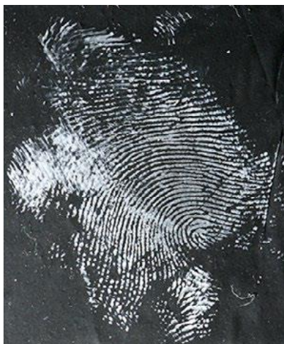
Figure 1.5 - Fingerprint developed with superglue fuming 2
