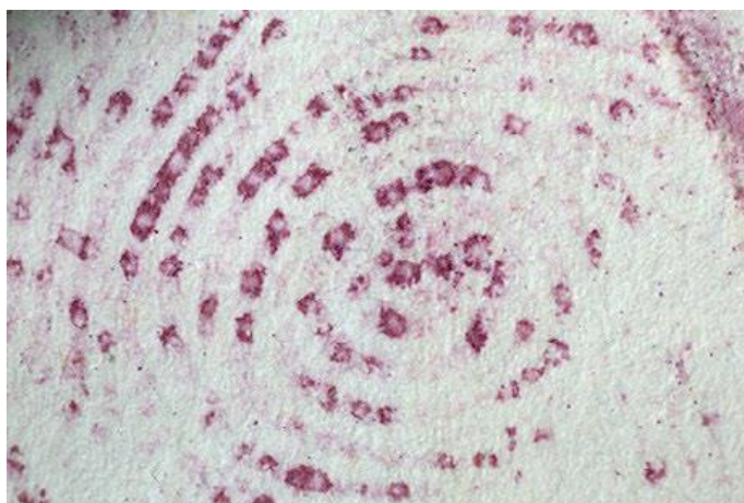
Figure 1.9 - Fingerprint developed with Ninhydrin
