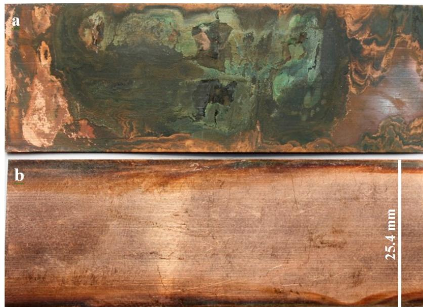
Figure 3.4: Optical image of outer and inner surface of the corroded tin-bronze reinforcing tape. The outer surface (a) is highly discoloured while the inner surface (b) shows only slight discolouration at the edges [3]
