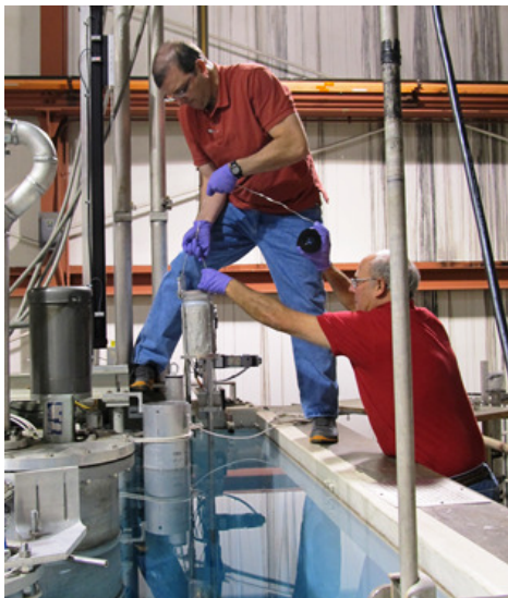
Figure 6. Experimental rig with the four bismuth telluride thermoelectric modules being loaded into the reactor pool.
