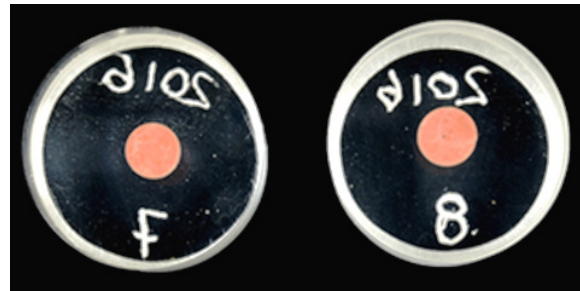
Figure 2. Sintered ~0.8 cm in diameter \text{CeO}_2 ceramic discs after mounting and polishing prior to the microhardness tests.
