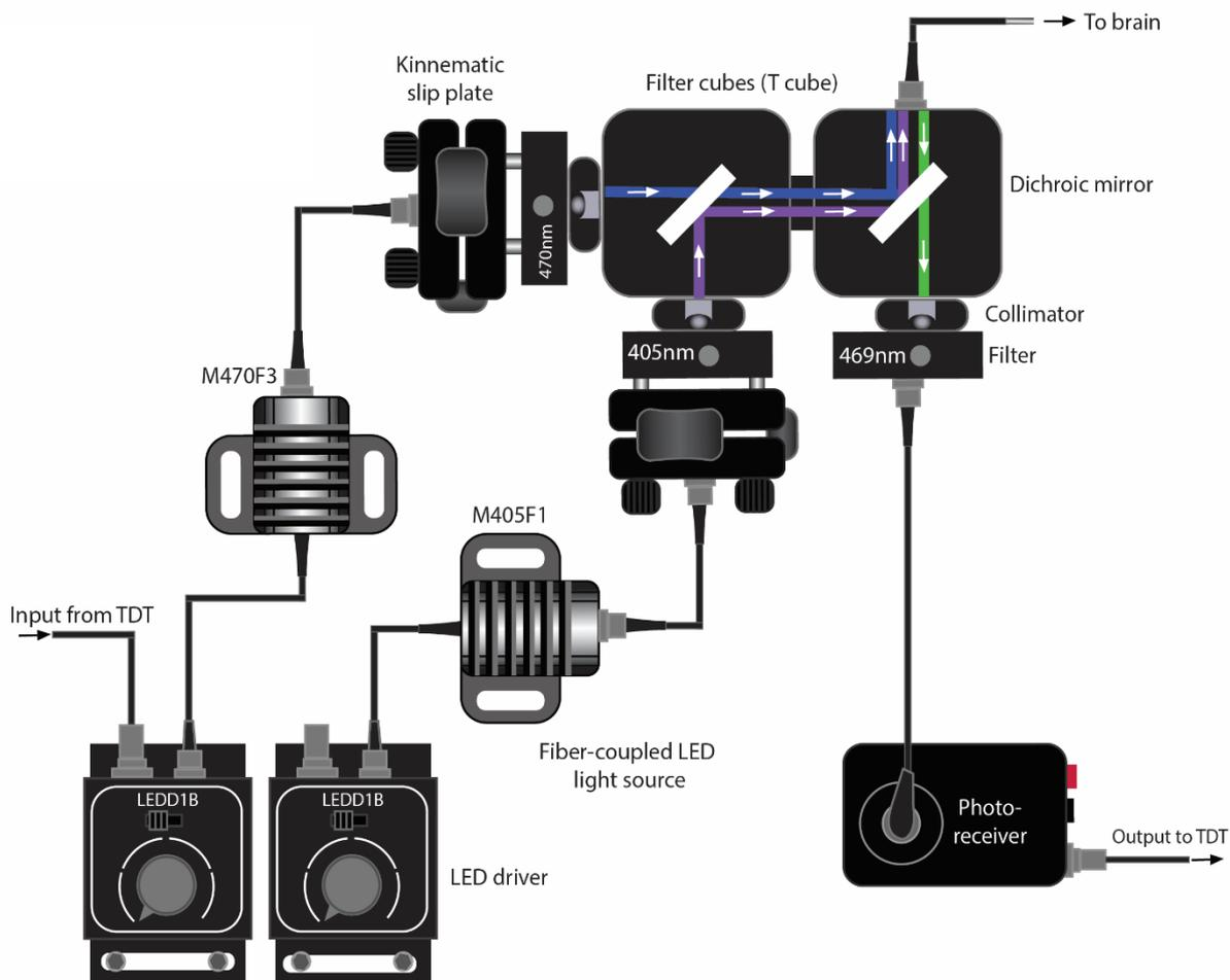
**Figure 4.4 – Fibre photometry set up**
