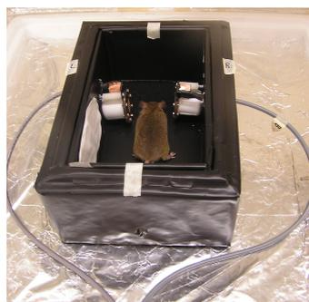
Figure 4- Ventilated chamber for acoustic traumatisation with ES1 speakers.
