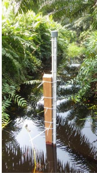
**Figure 2.29.** Example of gauge posts installed in a plantation channel
