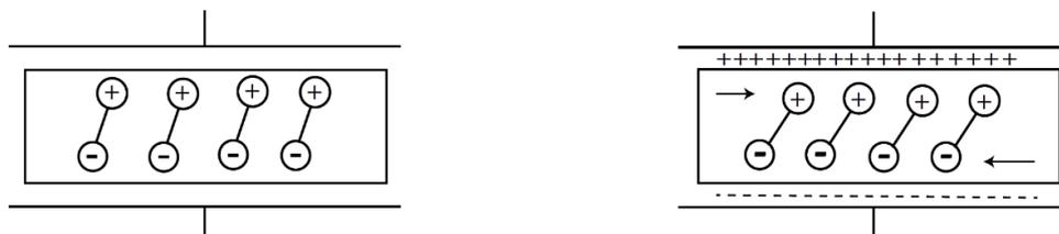
**Figure 2.6:** Schematic representation of the converse piezoelectric effect.
