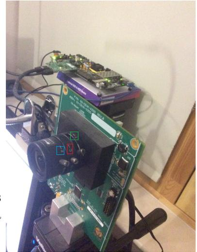
(c) The camera used for tracking data. The squares represent different tuning rings for picture quality.
