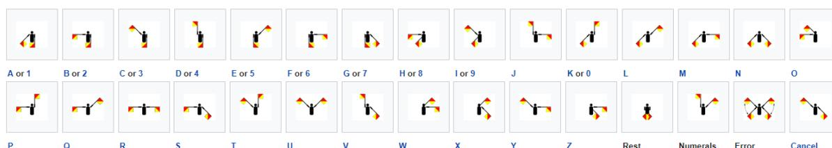
Figure 30: Representations of all thirty classes performed with two red and orange flags. These are all static positions except for Error which places both flags upright and is unique to the gesture’s motion without conflicting with other signals.
