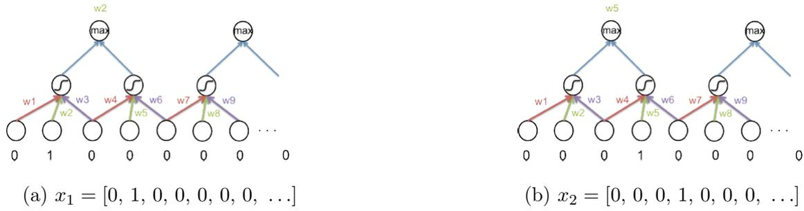
Figure 12: 1D representations of a white dot. Figure 12a is transformed by  $w_2$  and is two pixels away from Figure 12b, transformed by  $w_5$ . As the weights are equalised, the value after max pooling is unchanged. This property is called *Translational Invariance*.
