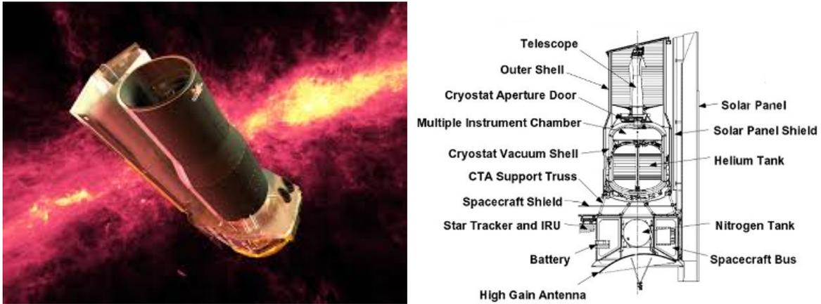
Figure 2.1: Left: Artist's impression of *Spitzer* Telescope, taken from <http://www.planetary.org/multimedia/space-images/charts/wise-telescope-design.html>. Right: Schematic illustrating main features of the *Spitzer* Telescope, showing the main housing and instruments. Image taken from <http://legacy.spitzer.caltech.edu/technology/overview.shtml>.
