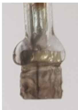
Figure S1. Voltammogram of grey material present on the working electrode after repeated cycling of PbSe, compared to the voltammograms of paint casted PbSe and elemental selenium (left), and an image of this grey coating (right).
