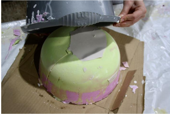
Figure k Removing the hardened plaster and mould from the bowl.
