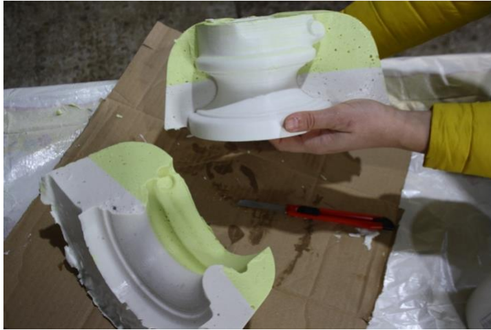
Figure g Prizing the alginate apart to reveal the negative impression.
