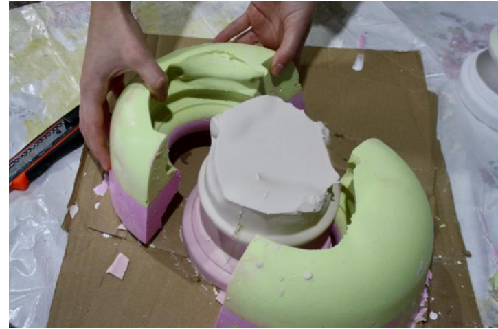
Figure l Carefully peeling away the alginate to reveal the plaster cast.
