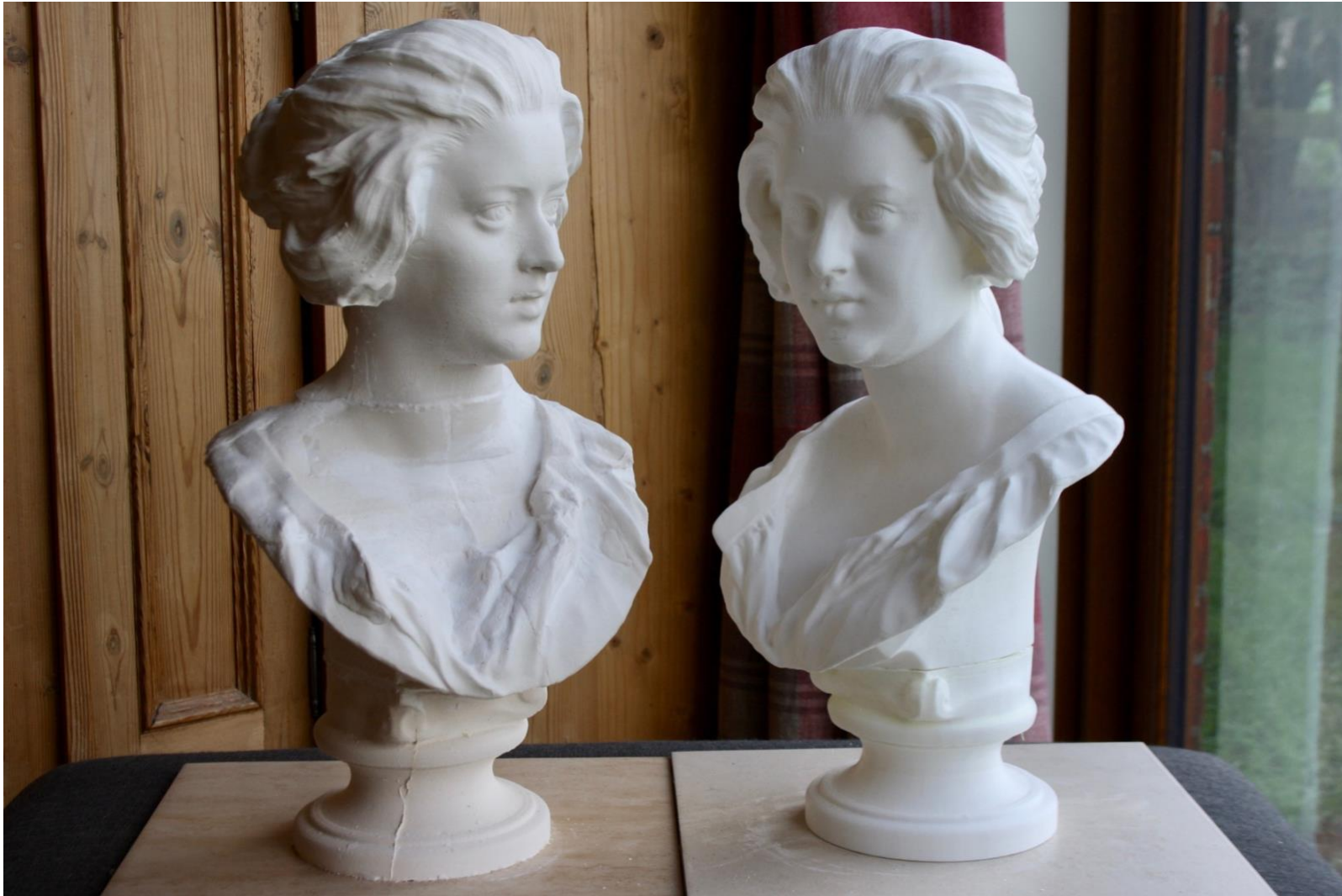
Figure n The completed plaster cast bust (left) and the 3D print that served as the model (right).
