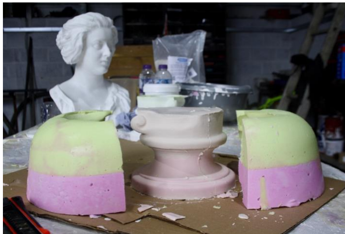
Figure m The plaster cast once removed from its alginate mould. The vertical line at the front of the base is a flashline, showing where the two alginate pieces had not sat flush together during the casting process.
