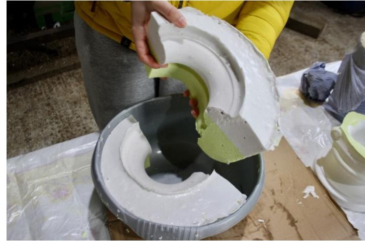
Figure h Placing the two pieces of alginate back inside the bowl.
