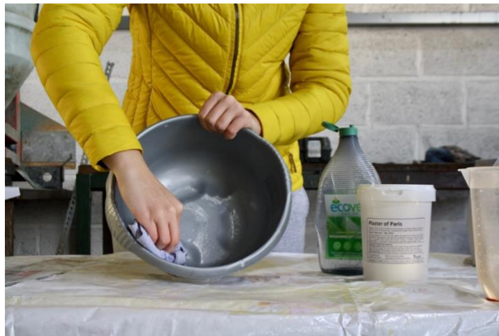
Figure a Coating the casting container in release agent.
