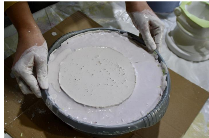
Figure j Rocking the bowl so that plaster fills every crevice.
