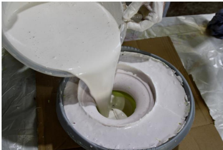
Figure i Pouring the Plaster of Paris into the negative mould
