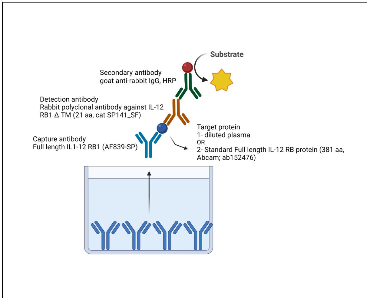
**Figure 5.1. ELISA model.** ELISA model to measure the plasma level of  $\Delta$ TM-IL-12R $\beta$ 1 peptide showing capture antibody, target protein, primary antibody, secondary antibody and substrate.
