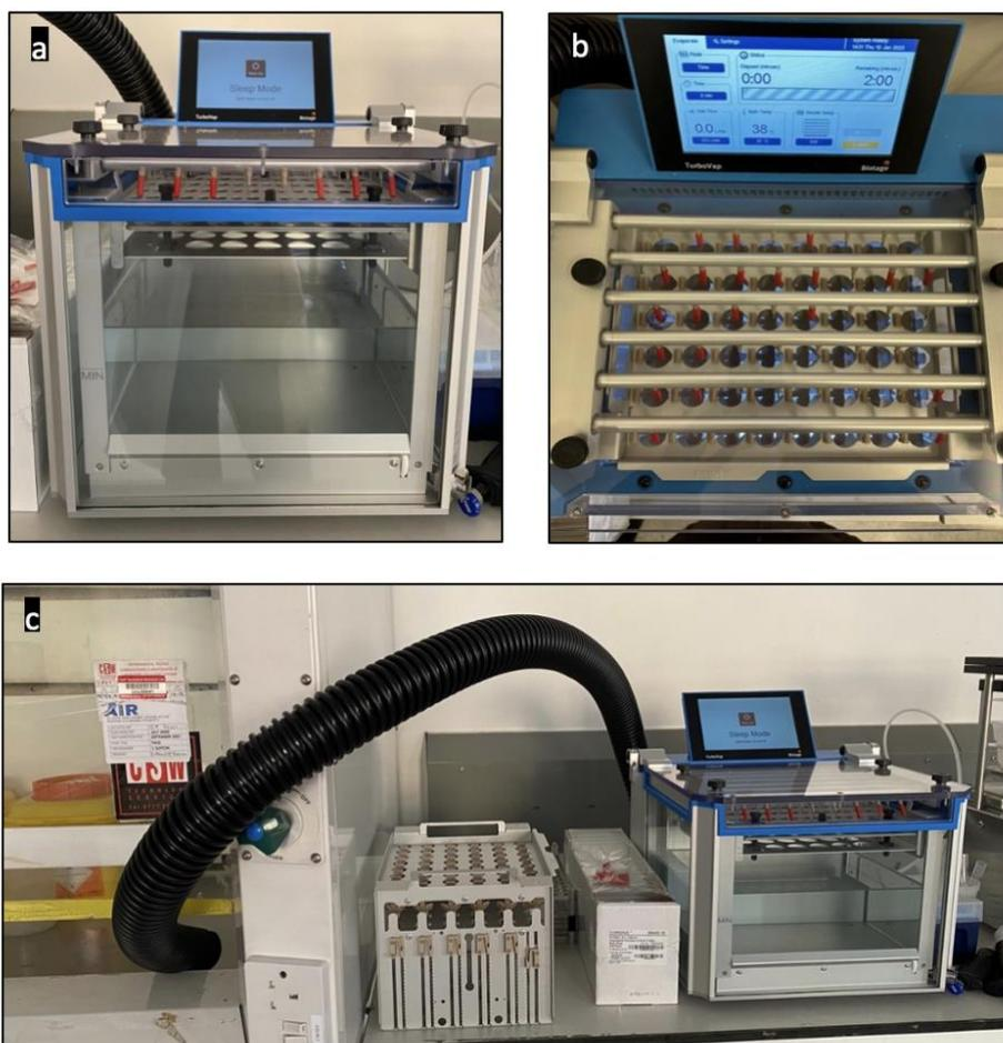
*Figure 2-6 The automated nitrogen evaporator system, TurboVap® LV system*
